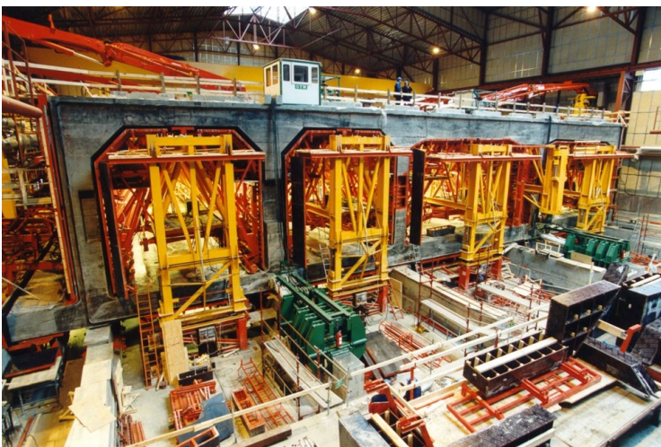
Casting of full-section by 22 m long tunnel segment in Oresund production factory
