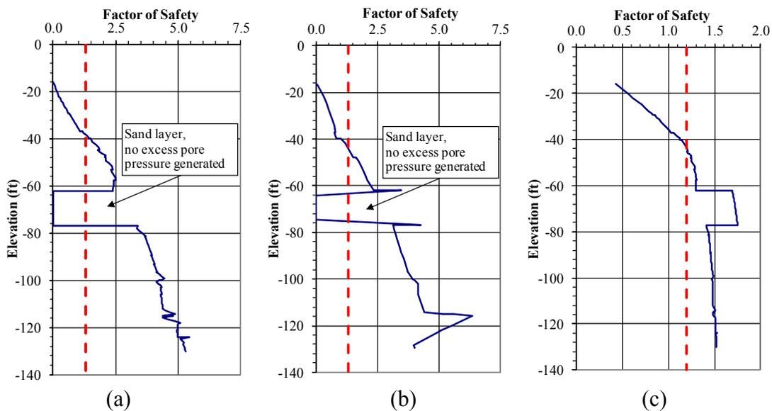
**Figure 6. Distributions of factors of safety based on the criteria for (a) exit gradient, (b) Terzaghi piping and (c) total weight heave.**
