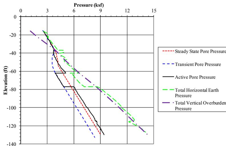
Figure 5. Comparisons of pore pressure with earth pressures.
