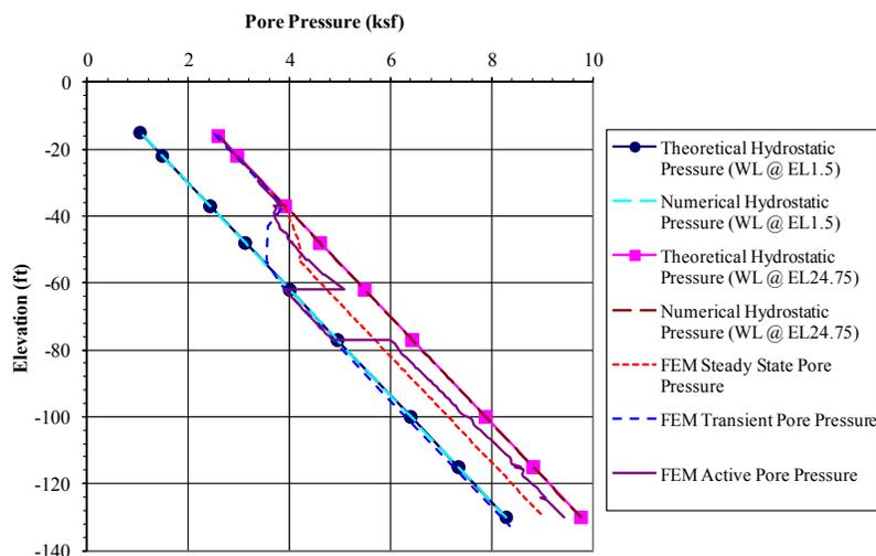
**Figure 4. Pore pressure distribution in front of a vertical concrete cylinder pile.**
