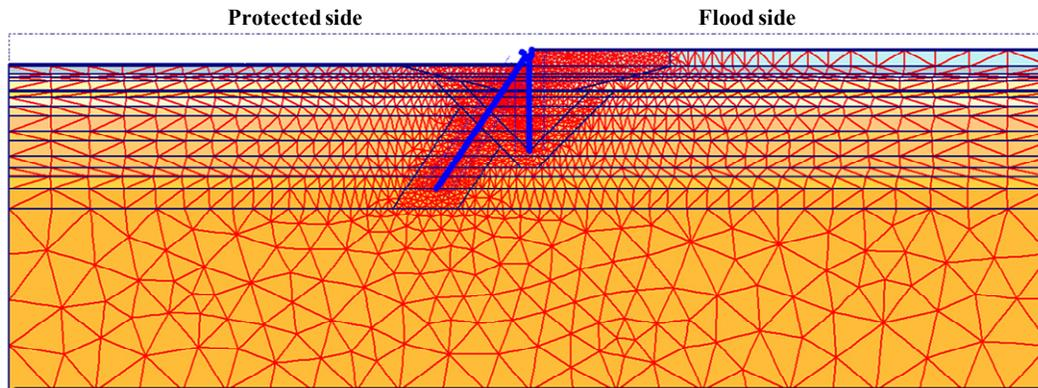
Figure 2. Mesh configuration for finite element seepage analysis.
