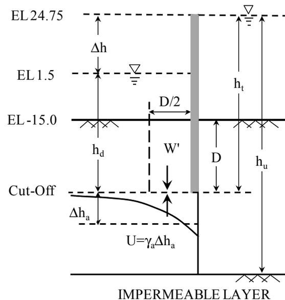
**Figure 1. Schematic diagram of seepage analysis.**
