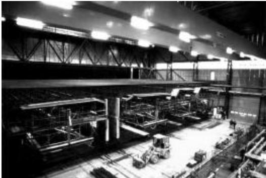
Figure 5 Completed 250 ton cages in buffer area waiting to be skidded into the casting cell
